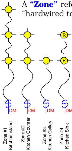
A **“Zone”** refers to a light fixture or group of light fixtures that are “hardwired together” and controlled by a switch or dimmer.
